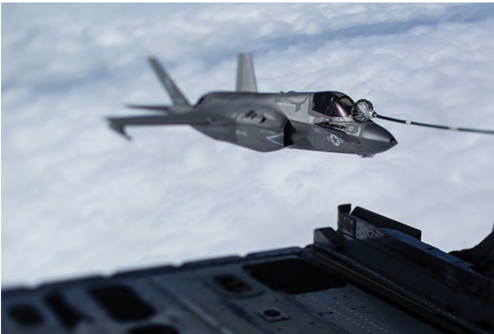
A U.S. Marine Corps F-35B Lightning II attack jet flies alongside a KC-130J tanker aircraft attached to a refueling drogue during an aerial refueling mission above the East China Sea, Oct. 23, 2018. Photo Credit: U.S. Marine Corps I Gunnery Sgt. T. T. Parish
